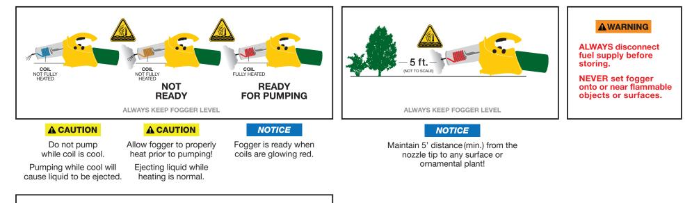
While heating, it is common for hot liquid to eject out of the nozzle. Always direct the nozzle in a safe direction.
