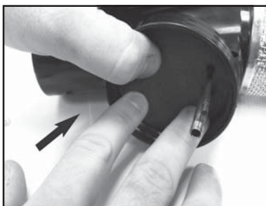
7. Push new gasket (161007) into place.
